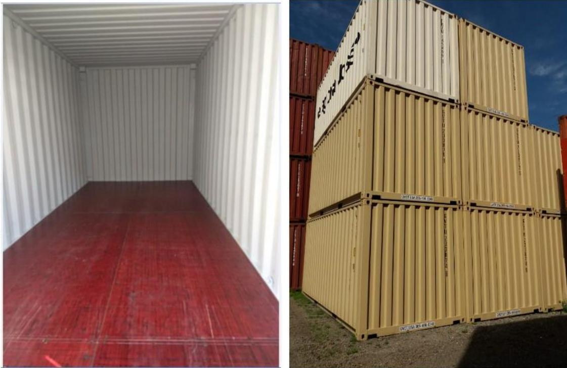
Figura 3 - Modelo Dry Standard / High Cube
